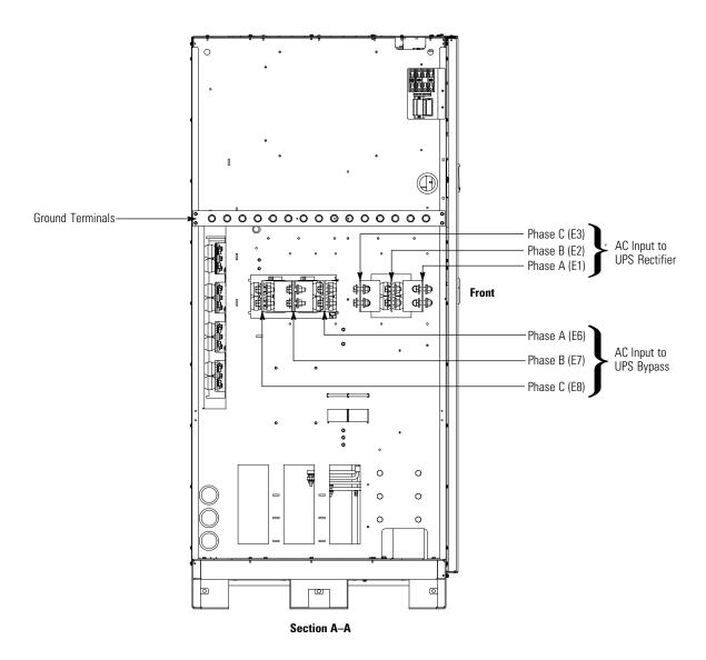
Figure 4-21. ISBM Section Power Terminal Detail AA – Common Rectifier Feed
